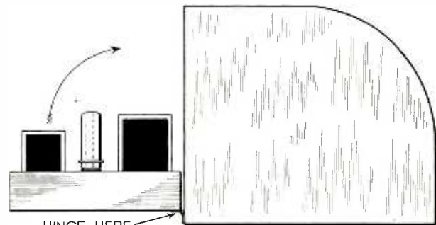
FIG. 2 Details of tilt-back chassis, for easy servicing.
