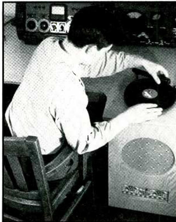
Cueing in a record. This view shows details of the bass reflex speaker inclosure, with lower port. Speaker cavity adjustment is covered in text.
