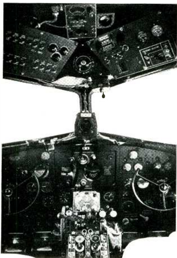
Cockpit of a Douglas DC-3 transport plane. At top of photo is the ADF tuning head. Frequency change switch at top right. In foreground is master radio panel and ADF Azimuth indicator.
